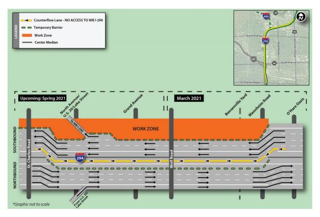
In 2021, the Tollway is beginning work to reconstruct and widen I-294 between Wolf Road and St. Charles Road, including rebuilding the bridges carrying I-294 over North Avenue, Grand Avenue and the Union Pacific Railroad and constructing the ramps that will connect I-294 to the new I-490 Tollway. Repair work is also scheduled on the Wolf Road Bridge over I-294.
