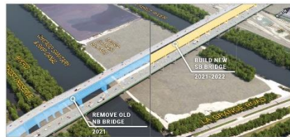
PHASE 2: Remove old northbound bridge and build new southbound bridge
