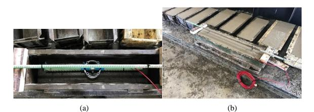
Figure 3.8 (a) Temperature beam with embedded gage and reinforcement bars; (b) the temperature compensation beams being cast.
