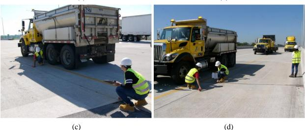
Figure 6.2 Research team conducting static truck loading test: (a) U of I research team (b) testing location with the team working on truck placement and data collection; (c) measurement of rear axle location; (d) measurement of front axle location.
