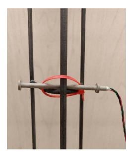
Figure 4-10. Strain gage secured to positioning chair with zip tie
