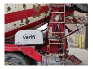
Figure 4-3. GCP applied technologies VERIFI® apparatus
