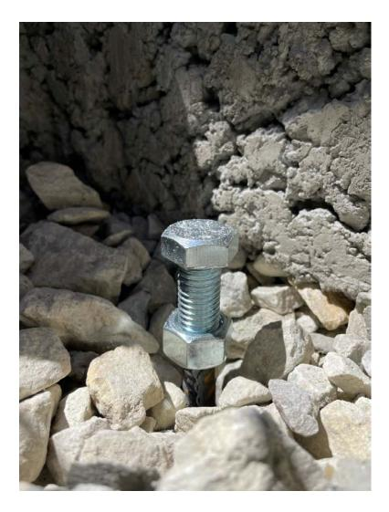
Figure 4-13. Reference point for lift off gage measurements
