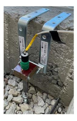
Figure 4-15. Lift off gage (LVDT) installed on the slab
