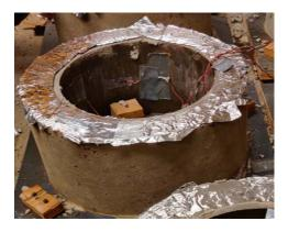
Figure 2-12. Restrained shrinkage measurement using ring test
