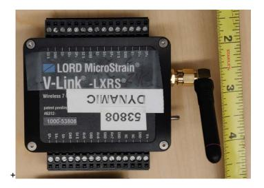
Figure 4-12. LORD MicroStrain V-Link wireless node
