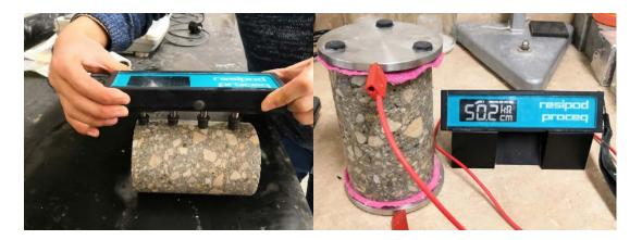
Figure 2-10. Testing apparatus for surface resistivity (left) and bulk resistivity (right)
