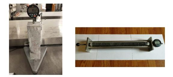
Figure 2-11. Shrinkage measurement (a) drying shrinkage and (b) autogenous shrinkage
