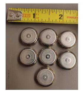
Figure 4-16. iButtons (temperature and relative humidity sensors)
