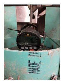
Figure 2-6. Surface settlement test
