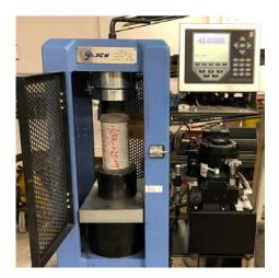
Figure 2-7. Test setup for compressive strength
