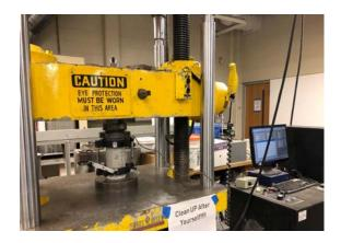
Figure 2-9. Testing set-up of modulus of elasticity
