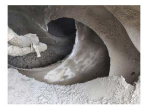
Figure 4-4. BASF SAP stuck to fins of mixing truck
