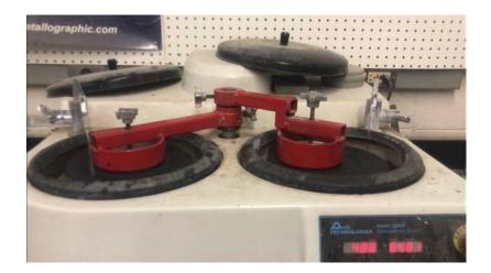
Figure 2-14. NANO 2000T grinder-polisher machine setup
