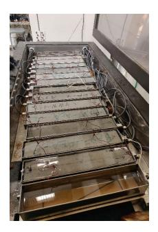
Figure 2-13. Test setup for frost durability
