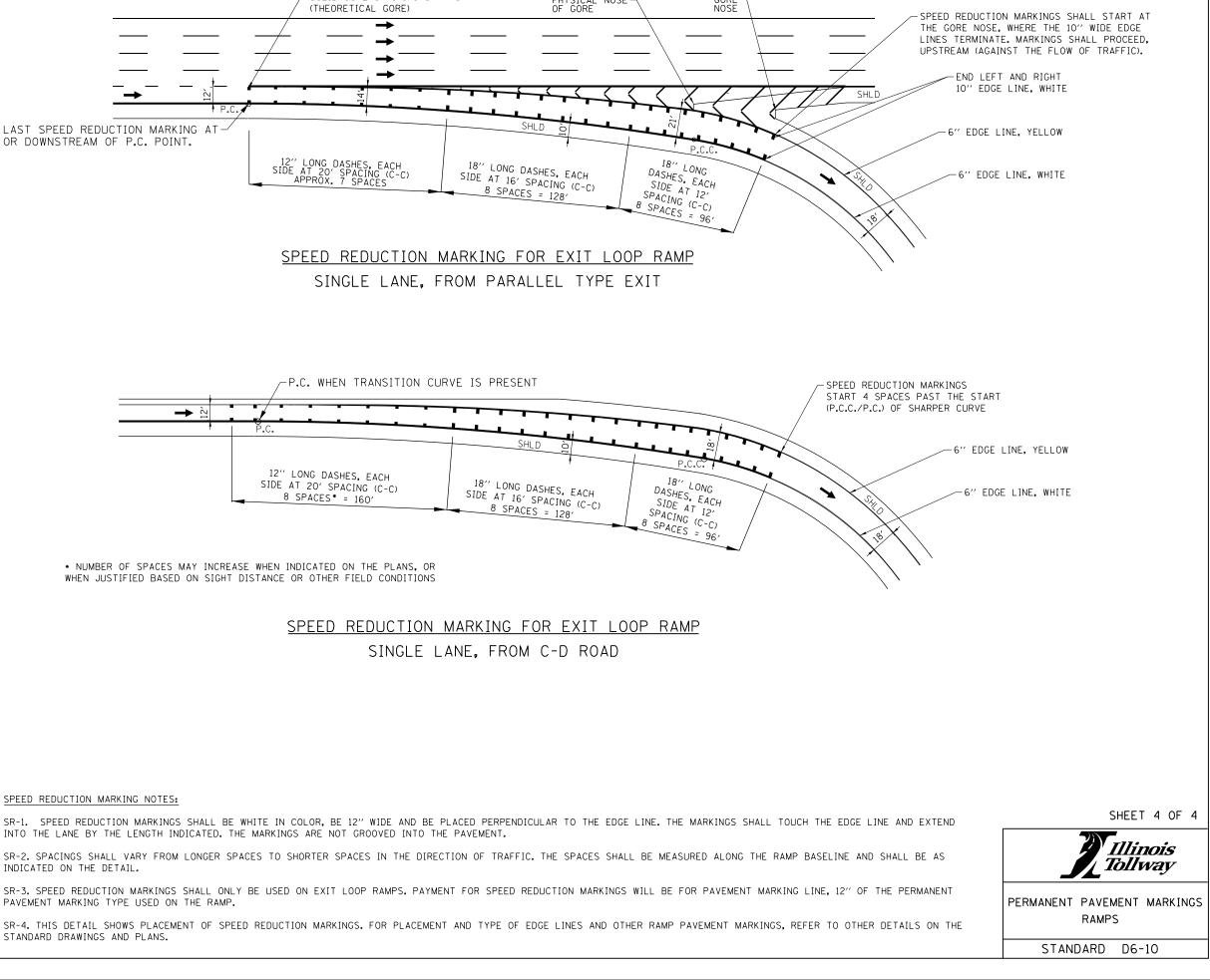
\* NUMBER OF SPACES MAY INCREASE WHEN INDICATED ON THE PLANS. OR WHEN JUSTIFIED BASED ON SIGHT DISTANCE OR OTHER FIELD CONDITIONS
