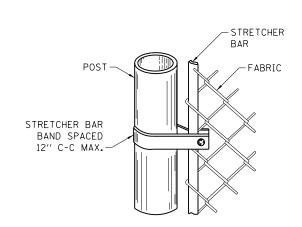
STRETCHER BARS SHALL BE GALVANIZED FLAT STEEL BAR NOT LESS THAN  $\frac{1}{4}$ " x  $\frac{3}{4}$ " AND THE STRETCHER BAR BANDS SHALL BE GALVANIZED FLAT STEEL BAR NOT LESS THAN 1/8"× 1" WITH A 3/8" GALVANIZED CARRIAGE BOLT.
