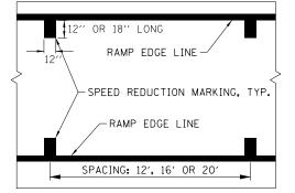
SPEED REDUCTION MARKING DETAIL
