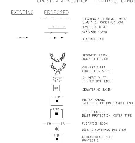
FLOTATION BOOM INITIAL CONSTRUCTION ITEM RECTANGULAR INLET PROTECTION TEMPORARY ROCK CHECK DAM
