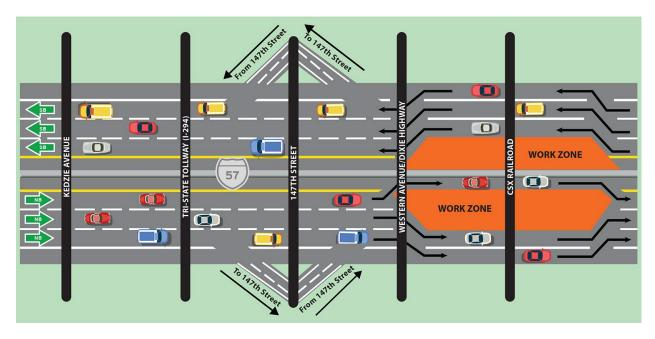
Tollway work is continuing to widen the CSX Railroad Bridge on I-57 as part of the I-294/I-57 Interchange Project. Pavement, and joint work will continue into 2023 at the I-57 bridge over the railroad. In addition, the Illinois Department of Transportation is resurfacing I-57 in this area.
