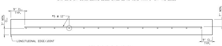
ONE MAT OF REINFORCEMENT SHALL BE FOR APPLICATION TO ALL STANDARD SLABS AND FOR ANY CUSTOM SLABS GREATER THAN 6 FT. LONGITUDINAL LENGTH TO BE OPENED TO TRAFFIC ONLY AFTER GROUTING IS COMPLETED.
