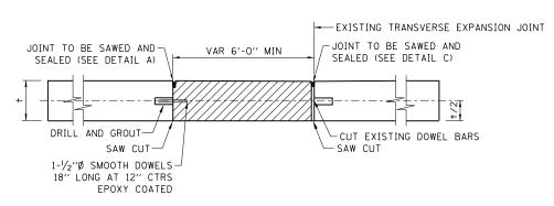
SECTION E-E REPAIR - FULL DEPTH, ONE LANE TRANSVERSE EXPANSION JOINT
