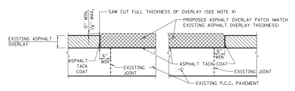
SECTION A-A ASPHALT OVERLAY REPAIR
