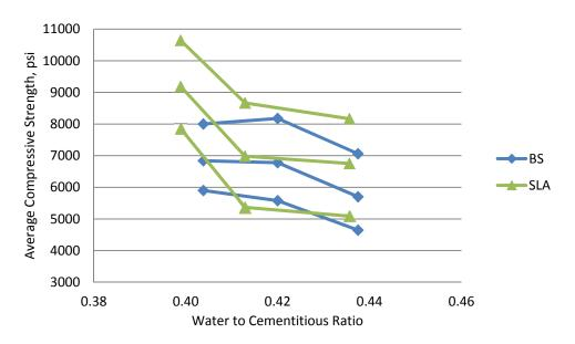
Figure 2: Average compressive strength of BS versus SLA
