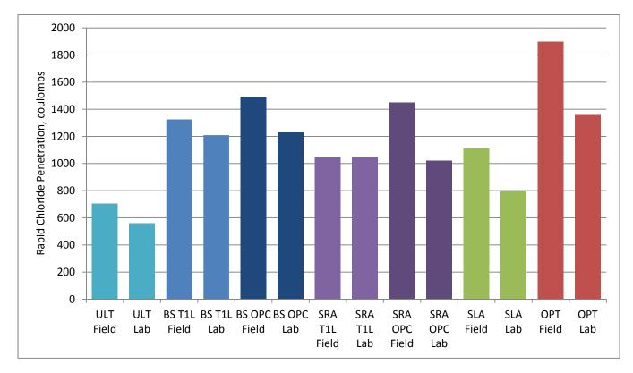
Figure 13: Rapid chloride penetration of field and lab mixtures
