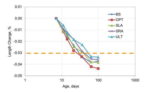
Figure 12: Drying shrinkage over time
