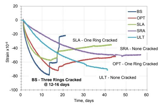
Figure 10: Restrained shrinkage over time
