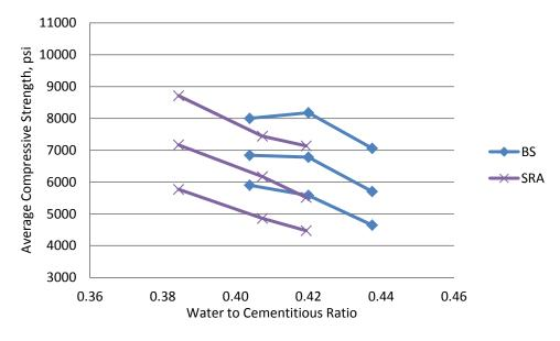
Figure 3: Average compressive strength of BS versus SRA
