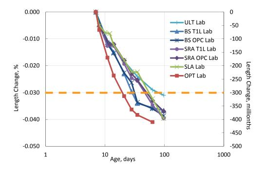
Figure 14: Drying shrinkage over time of Phase III lab mixtures
