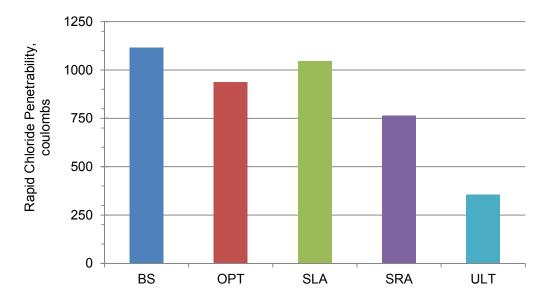
Figure 9: Rapid chloride penetrability (28 day accelerated)
