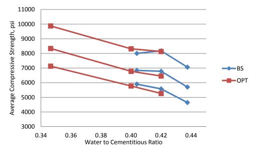
Figure 1: Average compressive strength of BS versus OPT
