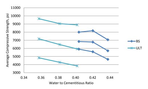
Figure 4: Average compressive strength of BS versus ULT
