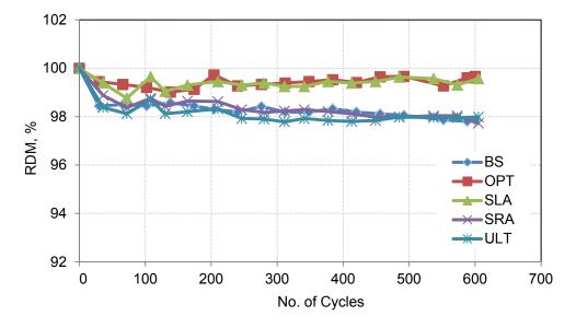
Figure 11: Freeze-thaw durability
