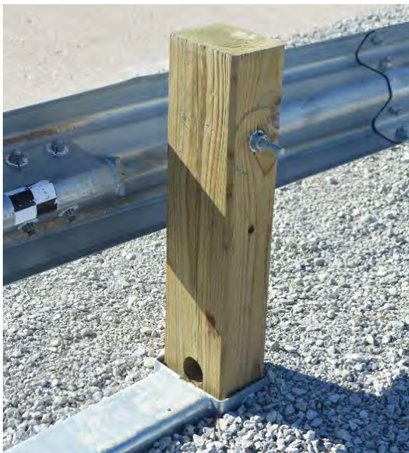
Figure 117. Upstream Anchor Damage, Test No. ILT-1
