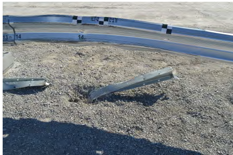
Figure 131. Post Nos. 12 through 15 Damage, Test No. ILT-2
