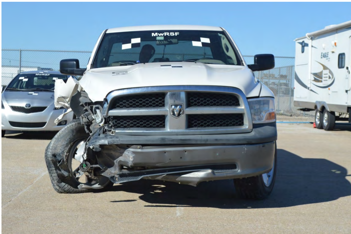
Figure 120. Vehicle Damage, Test No. ILT-1
