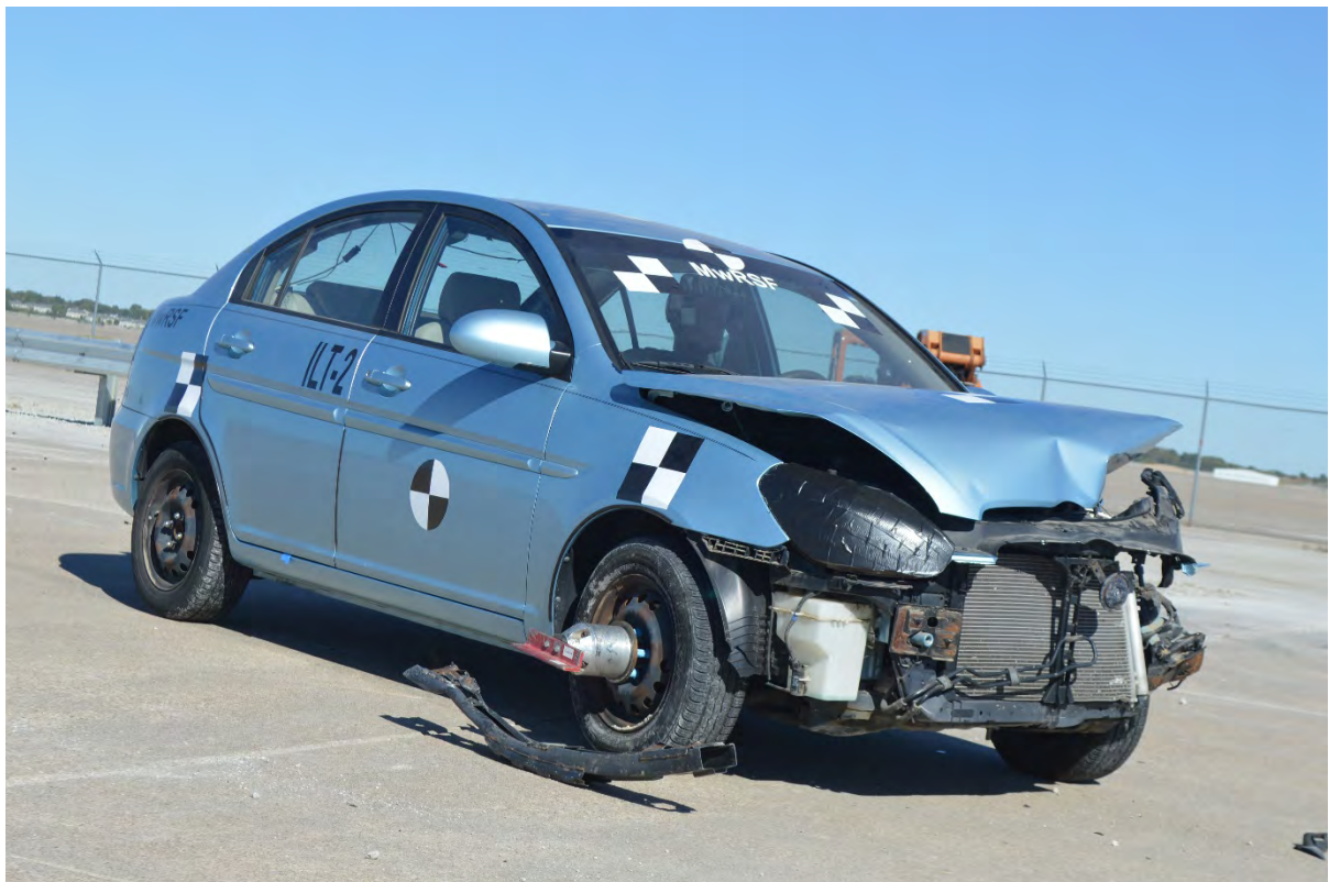
Figure 133. Vehicle Damage, Test No. ILT-2
