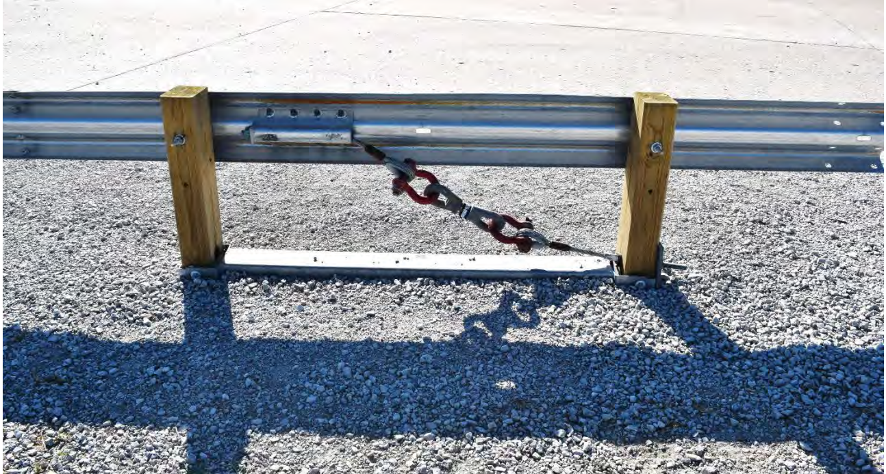
Figure 118. Downstream Anchor Damage, Test No. ILT-1
