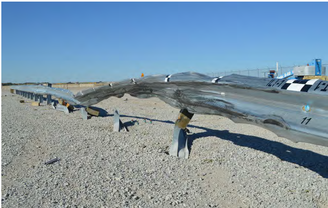
Figure 113. Midwest Guardrail System Damage, Test No. ILT-1
