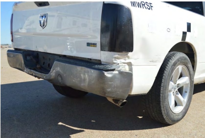
Figure 121. Vehicle Damage, Test No. ILT-1
