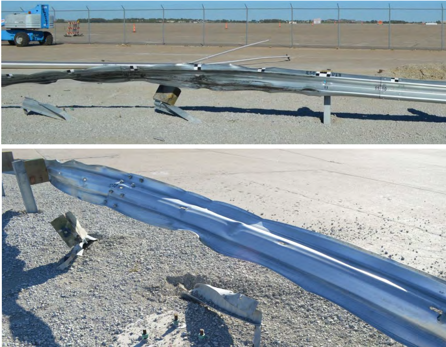
Figure 114. Rail Damage, Test No. ILT-1
