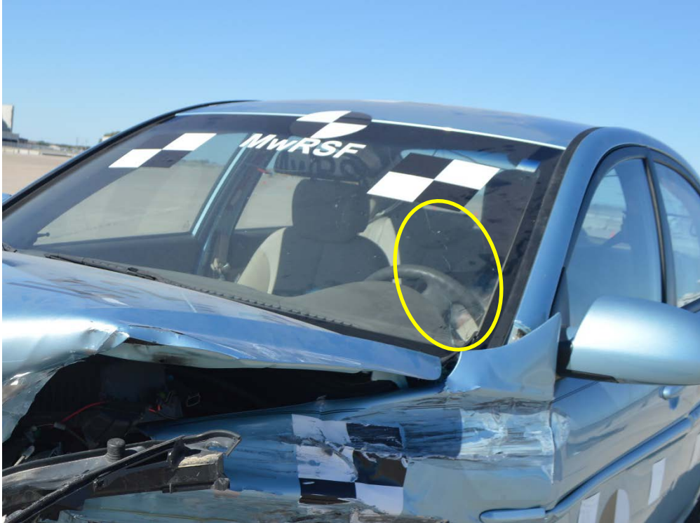
Figure 135. Vehicle Windshield Crack, Test No. ILT-2
