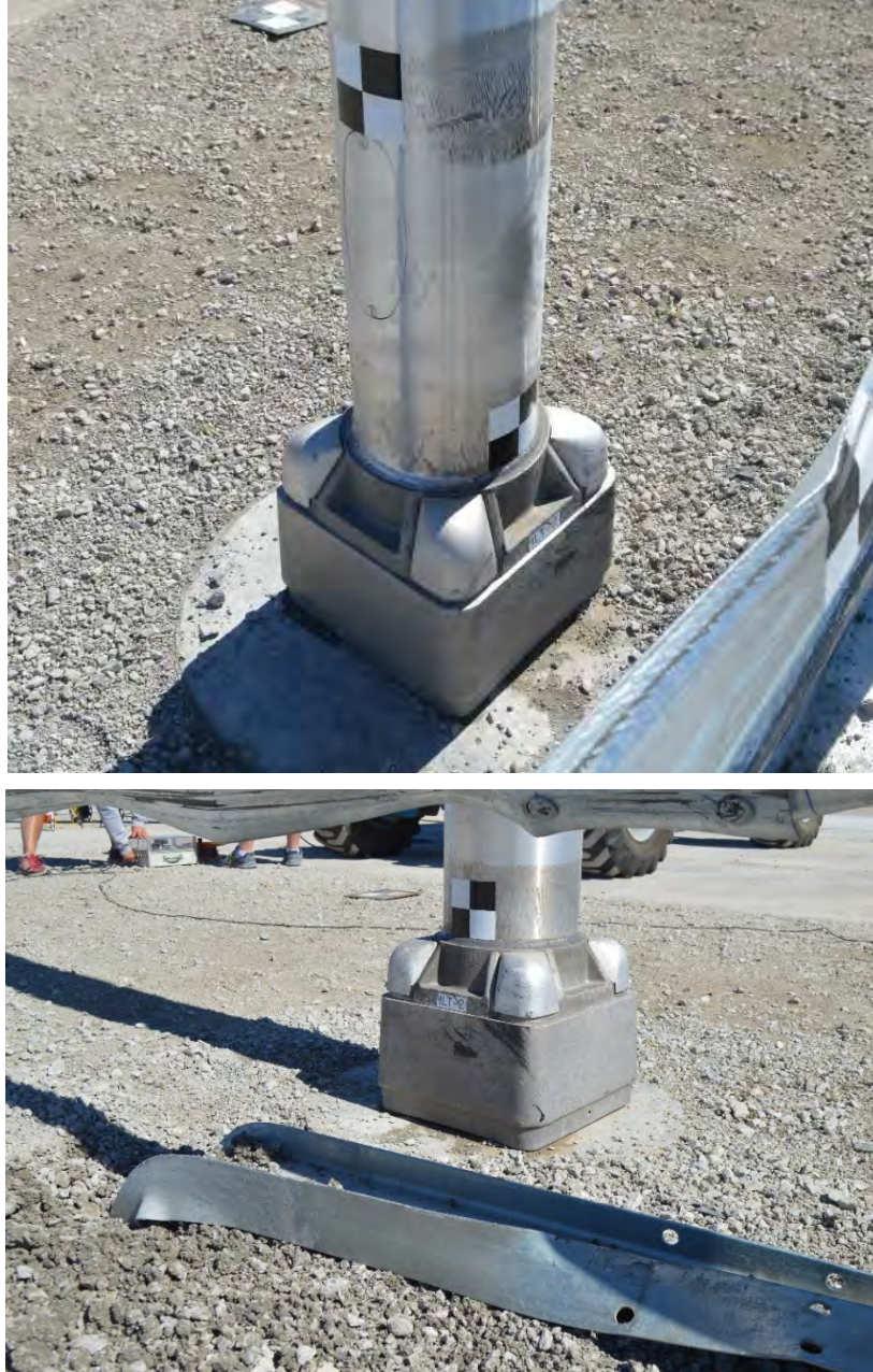
Figure 132. Pole Contact Marks, Test No. ILT-2
