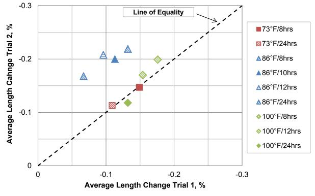
Figure 3-16 – Mortar Shrinkage Study – Trial 1 and Trial 2 comparison
