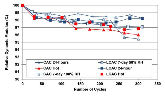
Figure 3-14 – F-T Testing - Relative Dynamic Modulus Results
