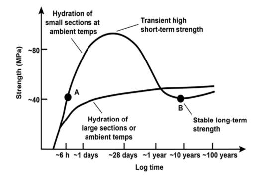
Figure 2-2 – Schematic Strength Development (Adapted from Campas, 1998)
