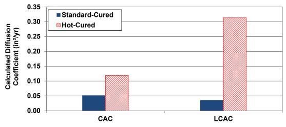
Figure 3-12 – Chloride Diffusivity Results
