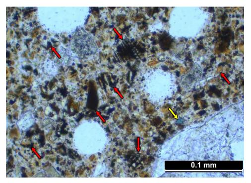
Fig. 2 Transmitted-light photomicrograph of Sample LCAC #2 Truck 9-6-16 in thin section, showing paste microstructure. Red arrows indicate residual calcium aluminate cement particles, comprised of various phases. Yellow arrow indicates particle of blue pleochroite phase. Plane-polarized light.
