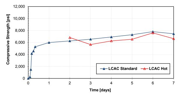
Figure 3-3 – Short-term LCAC Strength Development and Conversion
