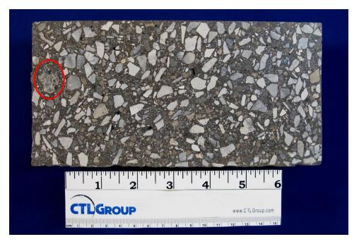
Fig. 1 Cut and lapped section of Sample LCAC Truck #2 9-6-16, struck surface at left. Section exhibits soft and powdery lump of unwetted cement and aggregate (red circle). Scale is in inches.
