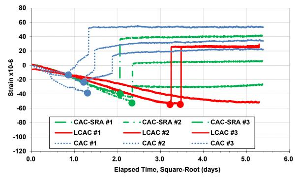
Figure 3-22 – Concrete Shrinkage Study – Restrained Shrinkage Test Results
