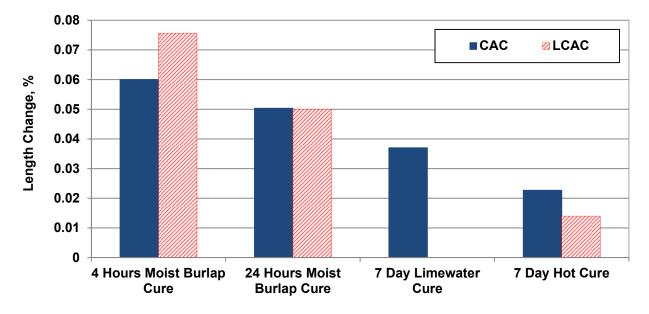
Figure 3-9 – Drying Shrinkage – CAC vs. LCAC3 3 - Volume Change Test Results
