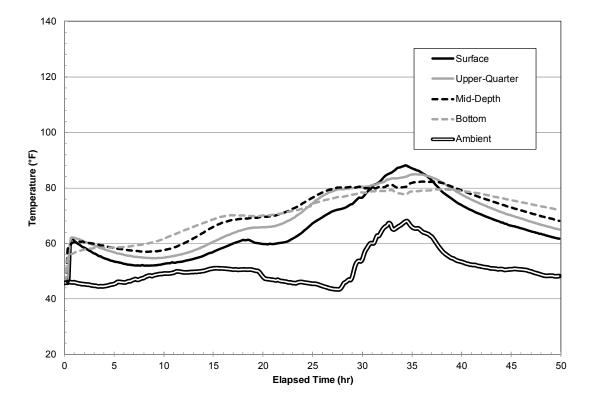
Fig. 22 – Patch center for non-accelerated placement of Patch 2.
