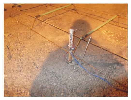
Fig. 26 – Layout of thermocouples at patch center (patch 3).
