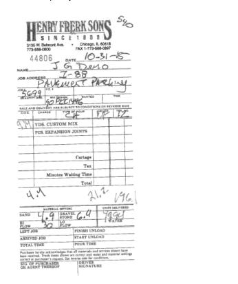
Fig. 14 – Patch 2 batch ticket for mixture with accelerator.
