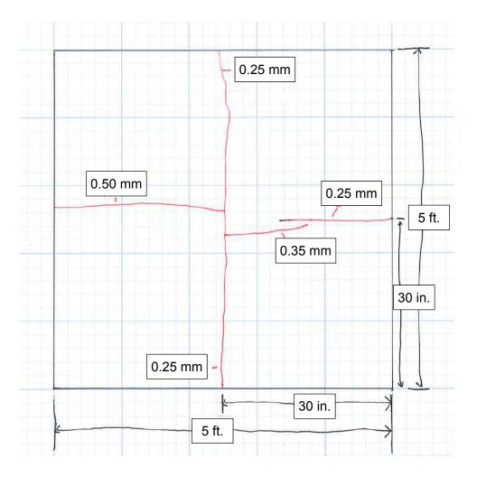
Figure 3-24 – I-294/North Avenue Repair – Crack Map at 36 hours
