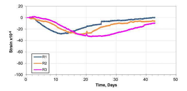
Figure 4-2 – Restrained shrinkage results – ALW4-T
