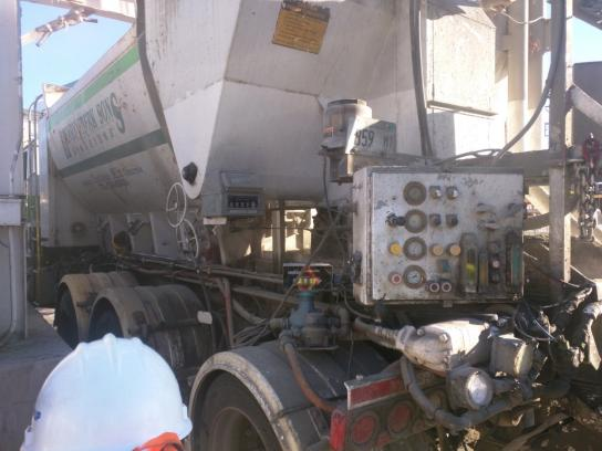
Figure 1 - Controls of Volumetric Mixer.
