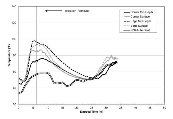
Fig.12 – Patch edge and corner temperature data for patch 1.
