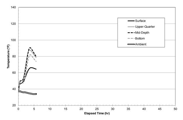
Fig. 35 – Patch corner temperature data for patch 3.
