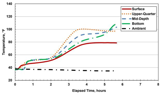
Figure 3-31 – I-294 Patch, Temperatures Center
