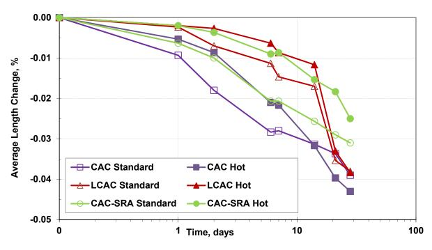
Figure 3-21 – Concrete Shrinkage Study – Drying Shrinkage Test Results
