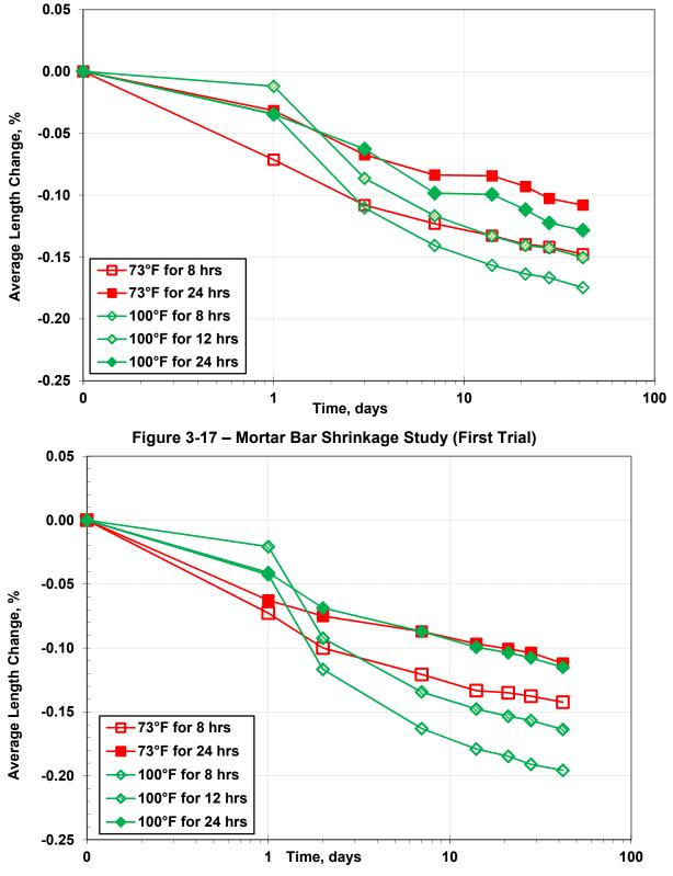
Figure 3-18 – Mortar Bar Shrinkage Study (Second Trial)
