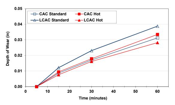
Figure 3-10 – Abrasion Resistance Test Results
