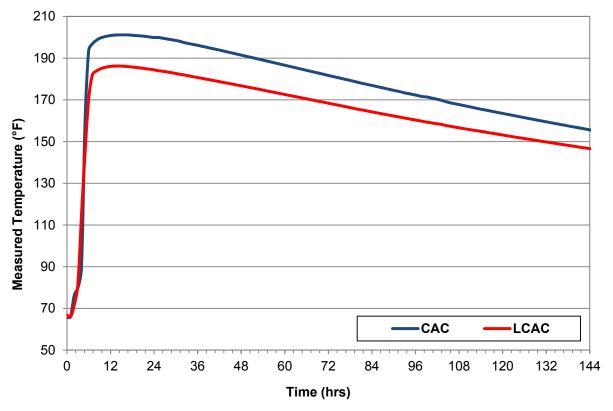
Figure 3-6 – CAC and LCAC Adiabatic Temperature Rise
