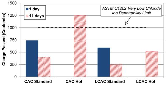
Figure 3-11 – Rapid Chloride Permeability Results
