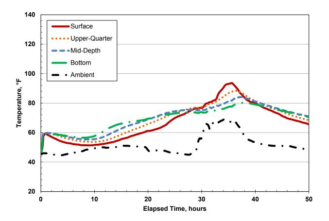
Figure 3-29 – I-88 Patch, Non-Accelerated LCAC (Edge Location)
