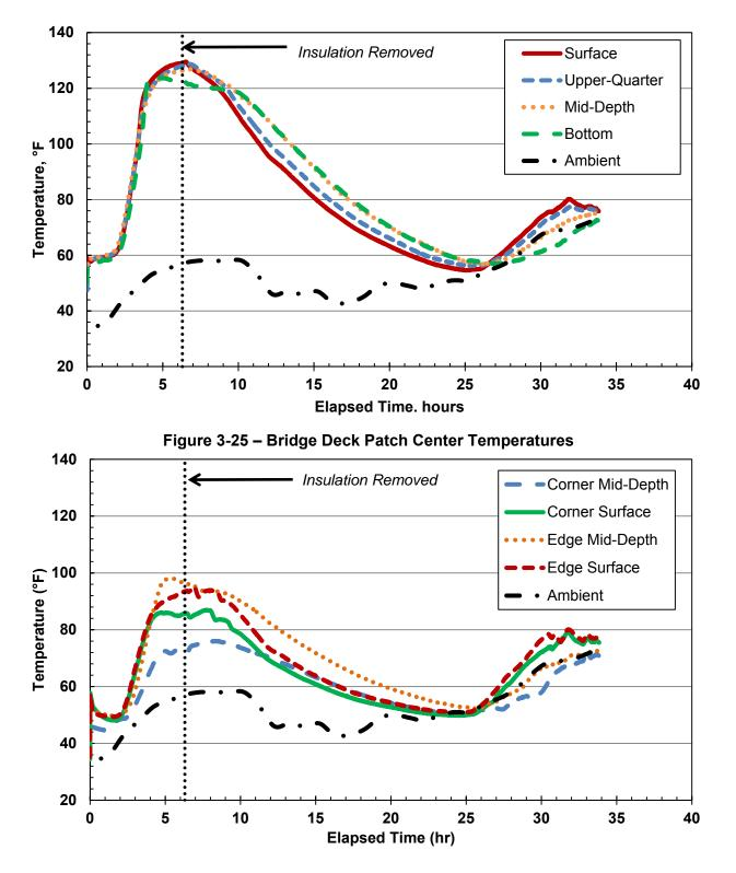
Figure 3-26 – Bridge Deck Patch Corner and Edge Temperatures
