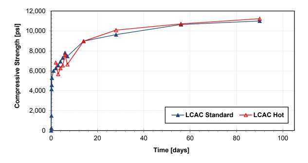
Figure 3-5 – Long-term LCAC Strength Development and Conversion
