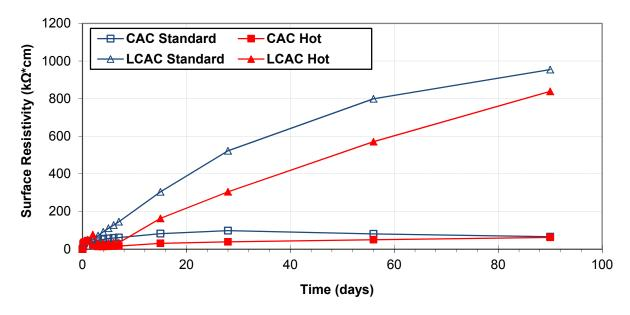
Figure 3-8 – Surface Resistivity, Long-Term
