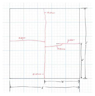
Fig. 10 – Crack map of patch 1.
