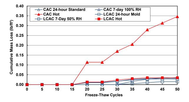
Figure 3-15 – Scaling Resistance Results
