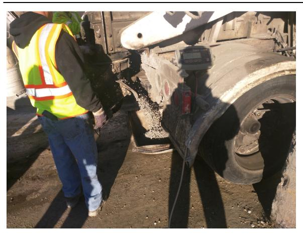
Figure 2 - Dispensing Aggregate for Calibration Procedure.
