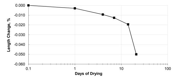
Figure 4-1 – Drying shrinkage results – ALW4-T
