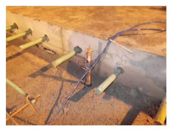
Fig. 27 – Layout of thermocouples at patch edge (patch 3).
