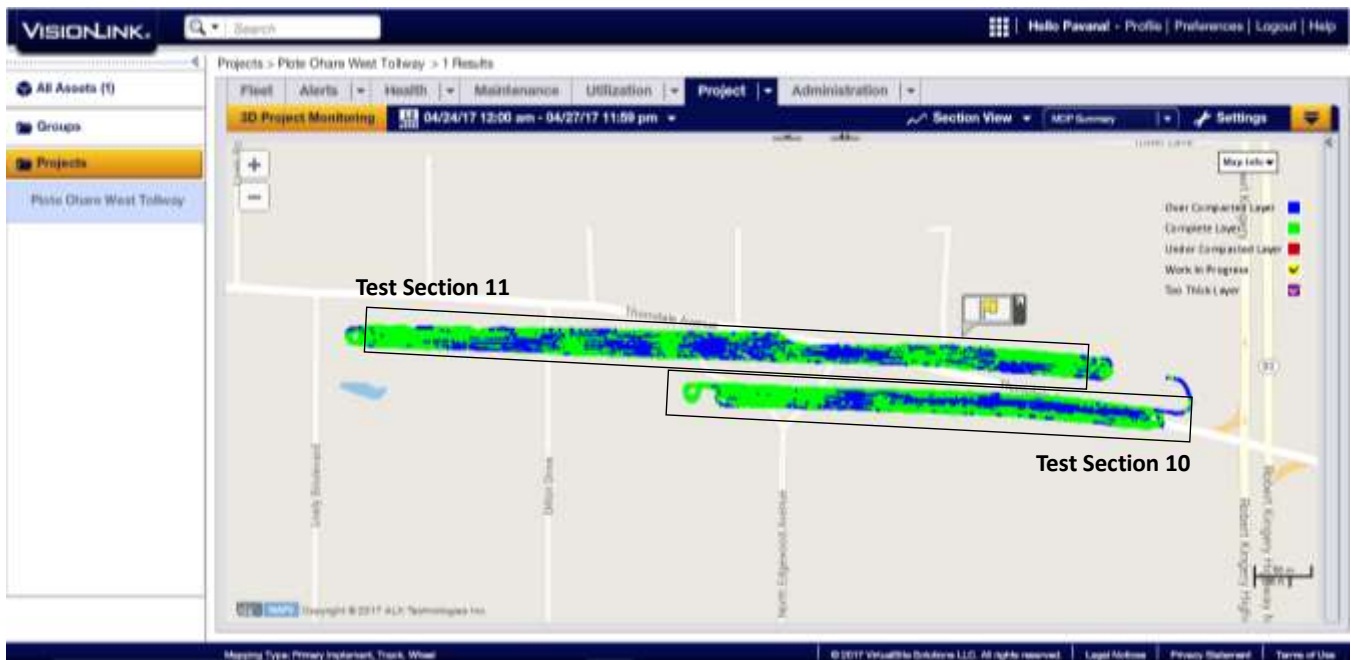
Figure 39. Screenshot of CMV and MDP* summary maps for TS10 and TS11 with PGE material.
