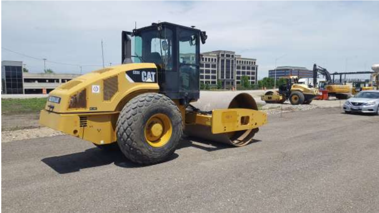
Figure 16. Caterpillar CS6 smooth drum roller with retrofit VIC system
