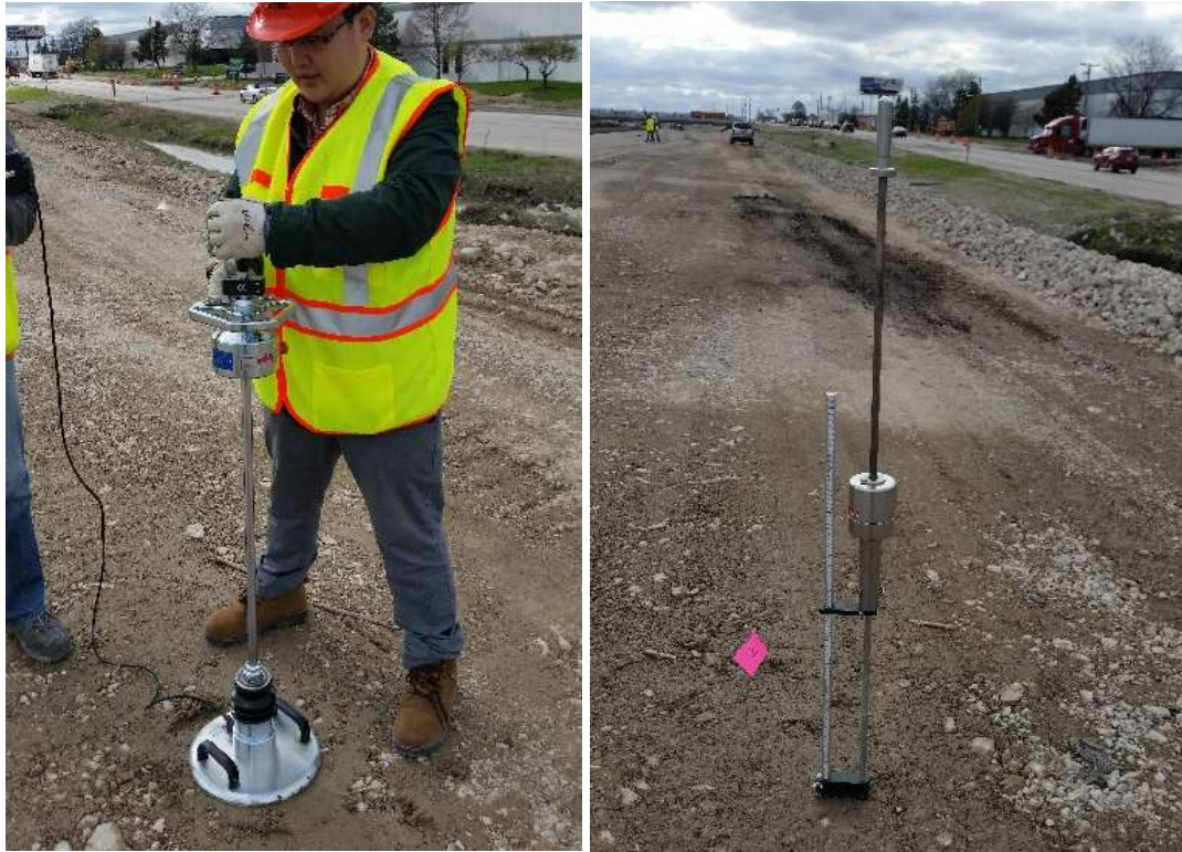
Figure 17. LWD (left) and DCP (right) testing on compacted CA6 capping layer.
