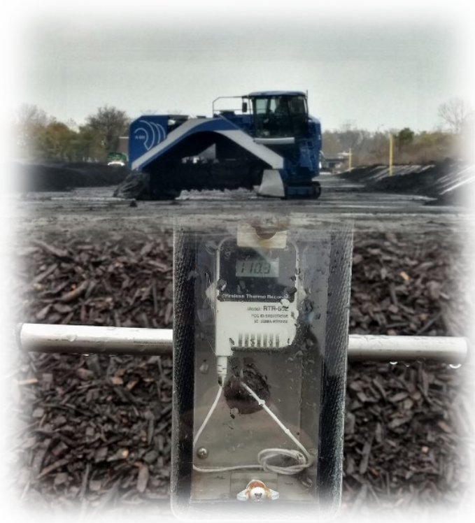
Figure 7 Auger used to turn compost piles at MWRD facility (above) and temperature monitor for active piles (below). Photo credit: Drew Monks, LUC.
