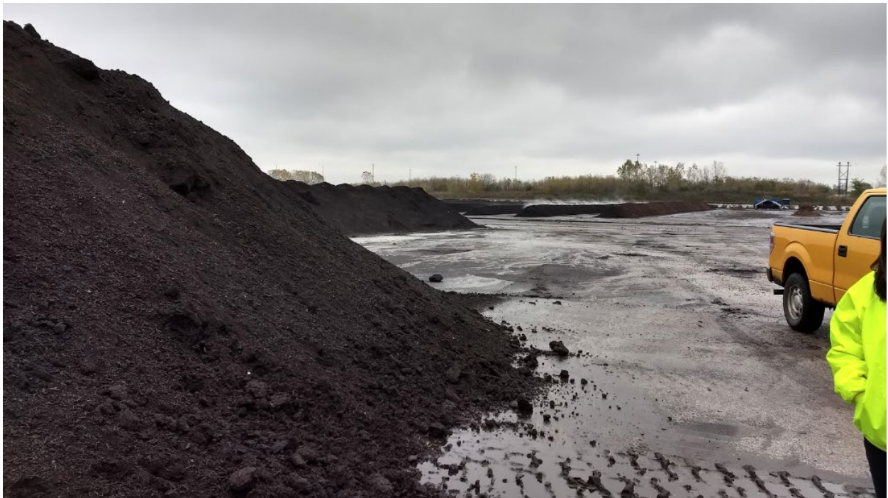
Figure 8 Finished compost product (foreground) with active steaming piles of compost (background) at the MWRD composting facility. Photo credit: Drew Monks, LUC.
