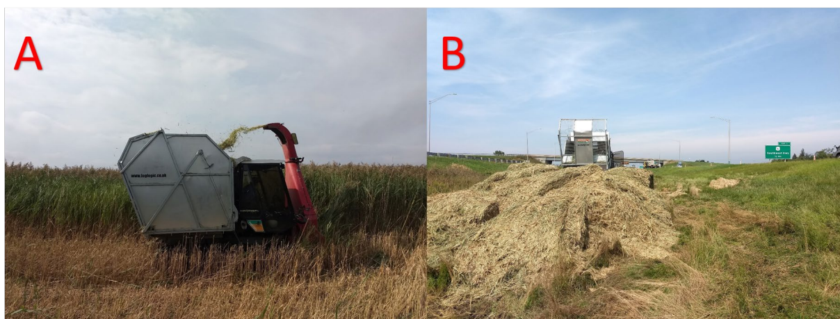
Figure 3 A) Softrak wetland harvester equipped with the Cut and Collect system harvesting Phragmites in basin 184, September 2019. B) Biomass pile waiting to be transported to MWRD, September 2019.
