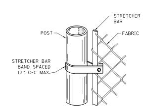
STRETCHER BARS SHALL BE GALVANIZED FLAT STEEL BAR NOT LESS THAN  $1\!\!\!/_4''~\times~3\!\!\!/_4''$  AND THE STRETCHER BAR BANDS SHALL BE GALVANIZED FLAT STEEL BAR NOT LESS THAN  $\frac{1}{8}$ "x 1" with a  $\frac{3}{8}$ " Galvanized CARRIAGE BOLT.
