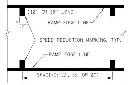
SPEED REDUCTION MARKING DETAIL
