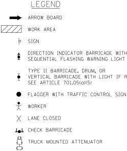
A. THE ADVANCE SIGNING SHOWN ON THIS STANDARD SHALL APPLY ANY TIME THE CONTRACTOR CLOSES ONE OR MORE LANES, OR IS REQUIRED TO SHIFT THE LANE ALIGNMENT. THE "ROAD WORK AHEAD" OR "ROAD CONSTRUCTION AHEAD" SIGNS, WORK ZONE PUBLIC INFORMATION SIGNS AND PORTABLE CHANGEABLE
