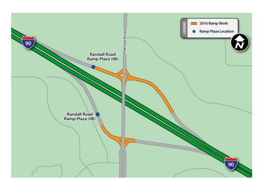
Weather permitting, beginning the week of May 23, construction is scheduled to start on all four interchange ramps. Work will begin by shifting traffic to the left to provide a work zone on the right for repairs. When work on the right side of each ramp is complete, traffic will shift to the right side to complete work on the left side of each ramp.
