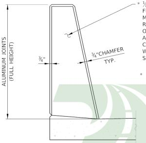
1/8" ALUMINUM P FULL HEIGHT MEETING THE REQUIREMENTS OF ASTM B209, ALLOY 3003-H14, COST INCLUDED WITH CONCRETE SUPERSTRUCTURE
