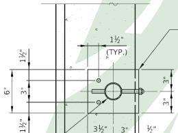
13"x6"x1/2" BENT OR WELDED BASE P W/3-3/4"Ø HOLES FOR  $\frac{1}{2}$ "Ø GALVANIZED EXPANSION ANCHORS W/WASHERS AND NUTS
