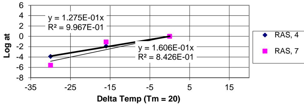
Figure 4. Time-temperature superposition shift factors.
