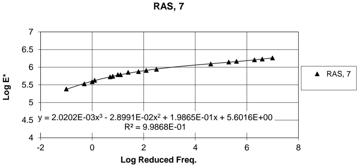
Figure 2. Dynamic modulus master curve for 7% air void samples.
