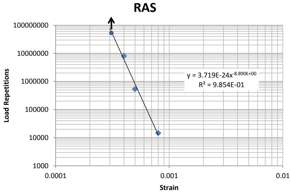
Figure 5. Fatigue curve for FRAP/RAS-SMA mixture.
