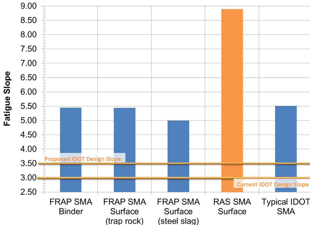
Figure 7. Fatigue slope comparison
