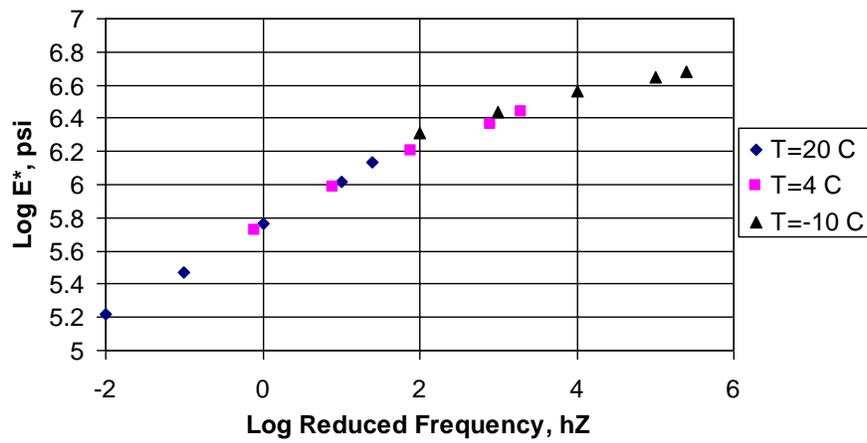
Figure 6. Dynamic modulus curve for IDOT District 1 SMA, 7% air voids.
