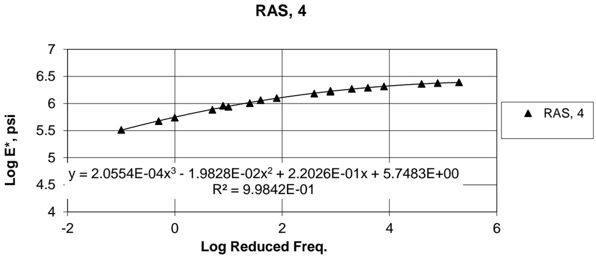
Figure 3. Dynamic modulus curve for 4% air void samples.
