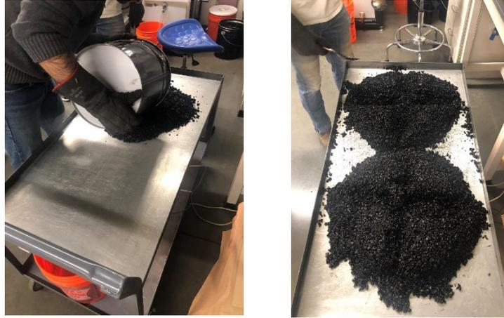
Figure 2-5. Splitting the bucket of mixture as per AASHTO R47
