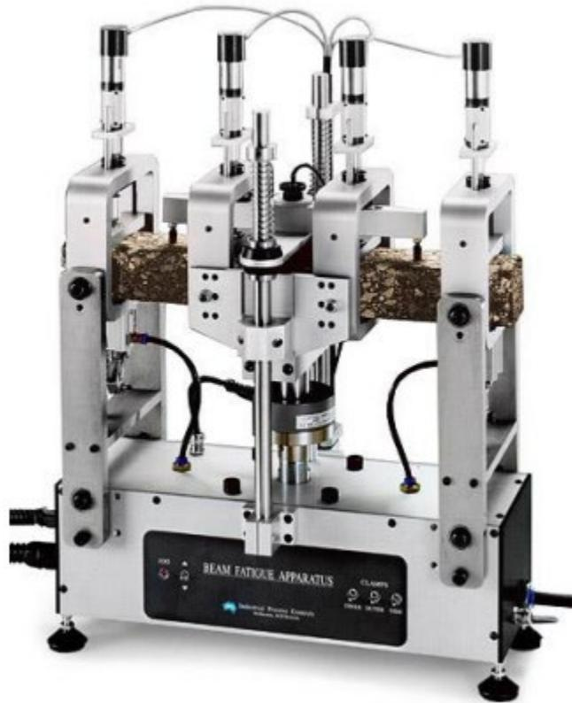
Figure A-4. Bending Beam-Fatigue Test (Saadeh & Eljairi, 2011)
