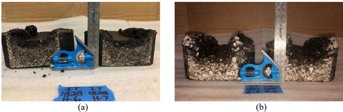
Figure 3-12. Tested samples after 20K pass at 50 °C. a) 1828 mix, b) 1834 mix
