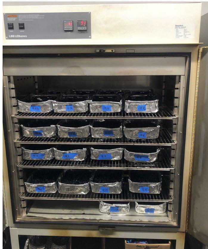
Figure 3-21. Aging the Tollway 2018 plant produced mixtures in oven at 95 °C for 6 days
