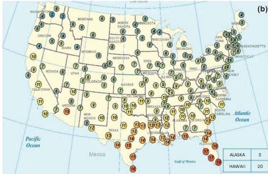
Figure 3-20. Required oven aging durations at 95°C to match level of field aging 6 mm below pavement surface for 8 years of field aging (Kim et al., 2018)
