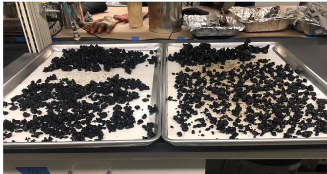
Figure 2-6. Preparing samples for theoretical maximum specific gravity ( $G_{mm}$ ) testing
