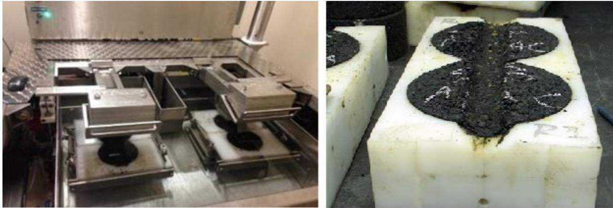
Figure A-7. Hamburg Wheel Tracking Device a) Test running b) After test (W. G. Buttlar & Rath, 2017)
