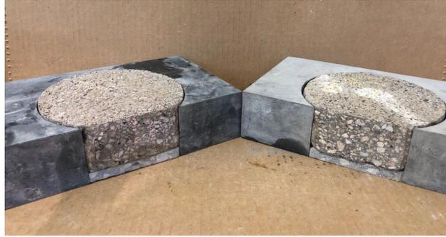
Figure 5-7. Hamburg samples with 12mm PCC shims placed below asphalt specimens
