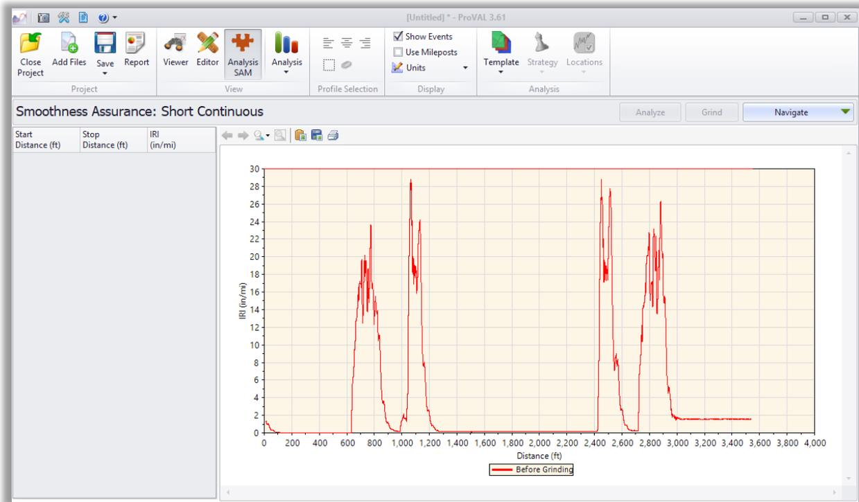
The peaks on the smoothness assurance graph are below the 30 in/mi IRI threshold and hence meets RDC requirements for mainline.
