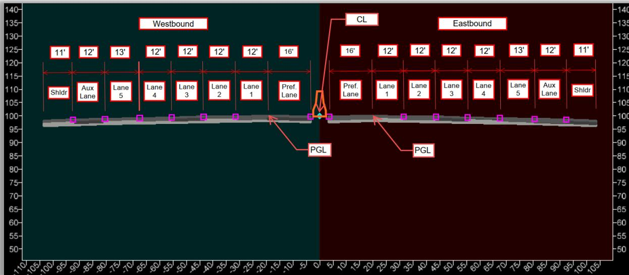
Go to *Corridor Modeling* from *Civil Tools* and select the *Superelevation Editor*, click on the Superelevation Editor Boundary (See Corridor Model Plan View figure in Section 2.1.1)
