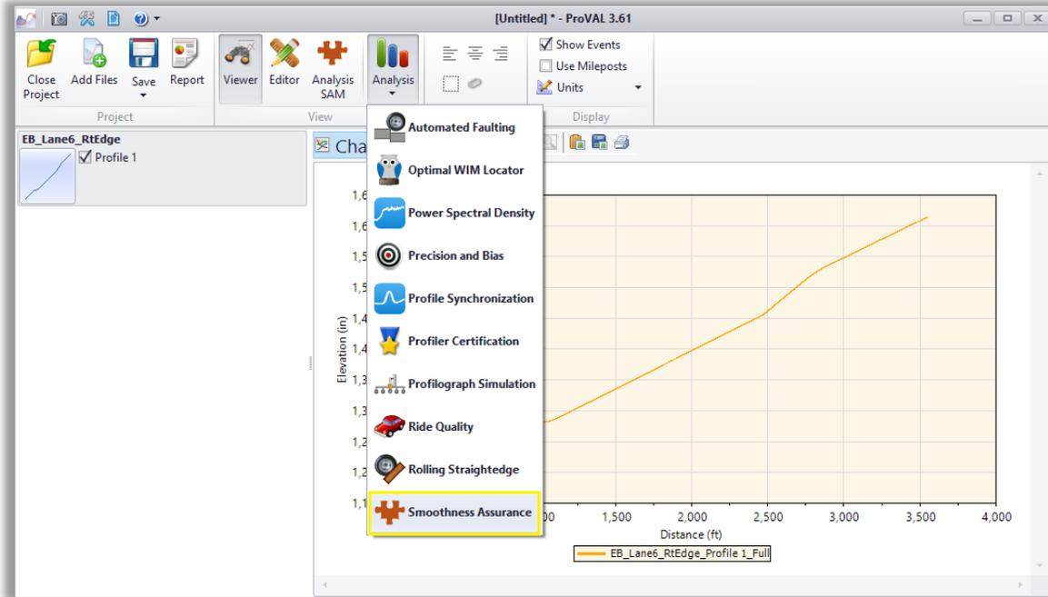
A *Smoothness Assurance* window appears. Adjust the IRI Threshold to be 30 in/mi (mainline roadway). (The Threshold for a ramp is 50 in/mi). Select the *EB\_Lane6\_RtEdge*, then click **Analyze**.
