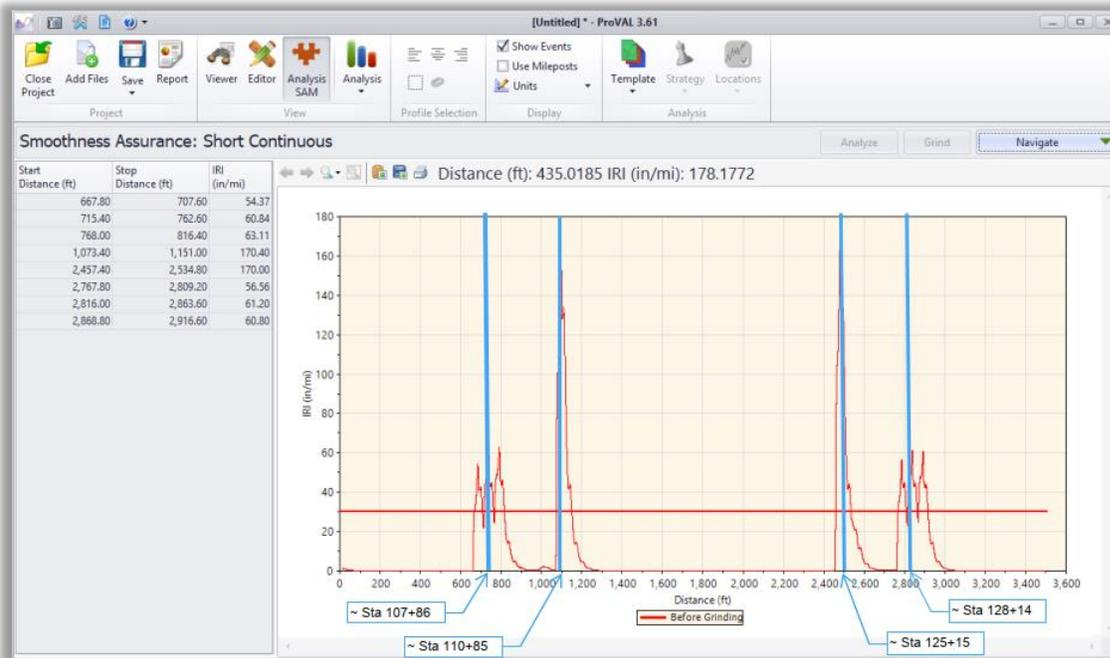
These stations in the *Superelevation Editor* in Geopak SS4/SS10 align with the locations of the superelevation break points. Vehicles traveling at these locations would experience undesirable bumps at the breaks. This supports the importance of incorporating vertical parabolic curves at superelevation breaks to ensure pavement smoothness for vehicles.
