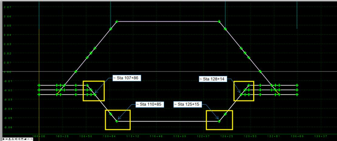
After repeating the steps of exporting the profile geometry and performing the Smoothness Assurance Module for this scenario, the ProVAL results yield peaks well in excess of the 30 in/mi IRI at STA 107+86, STA 110+85, STA 125+15, and STA 128+14, which correspond to the SE transition breakpoints in the above *Superelevation Editor*.
