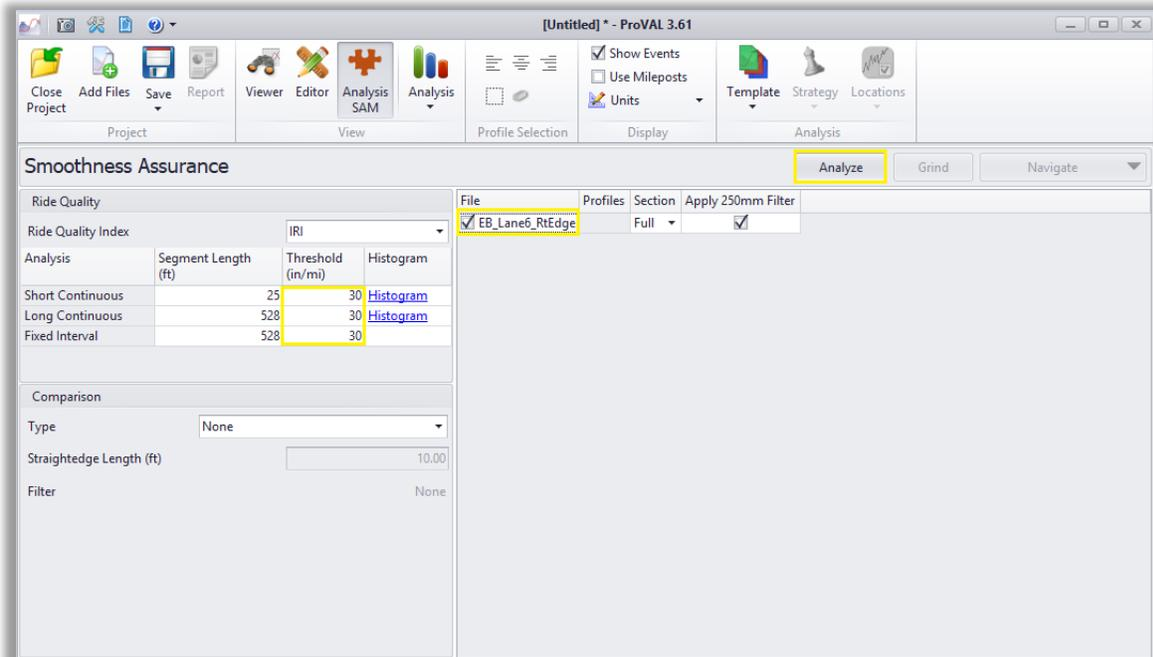
An analysis will run, which will activate the *Navigate* selection. Select **Short Continuous** from the *Navigate* drop down menu. The *Short Continuous* analysis indicates localized roughness and navigates locations of bumps in the pavement. The *Long Continuous* analysis evaluates the general condition of the pavement.
