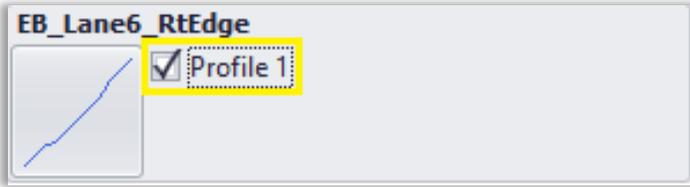
The chart will display the lane edge profile with Distance (ft) along the x-axis and the Elevation (in) along the y-axis.
