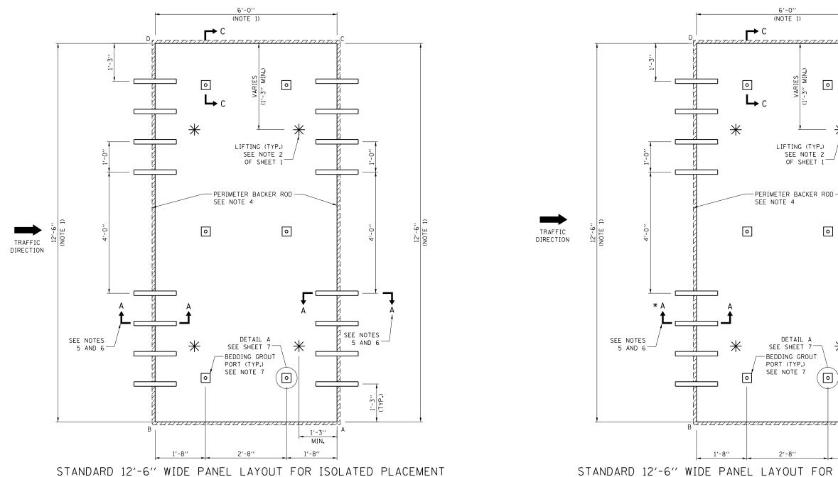
WITH EMBEDDED DOWELS FOR PRECUT WIDE MOUTH SLOTS IN ADJACENT PAVEMENT
