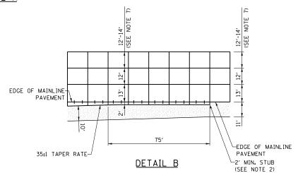
JOINTED PCC RAMP ADJACENT TO JOINTED PCC MAINLINE PAVEMENT
