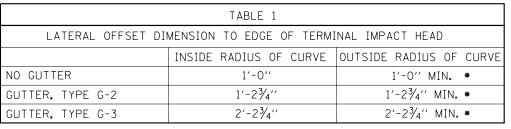
(\*) OFFSET DISTANCE WILL VARY BASED ON RADIUS OF HORIZONTAL CURVE AND THE TERMINAL BEING INSTALLED IN A STRAIGHT LINE.
