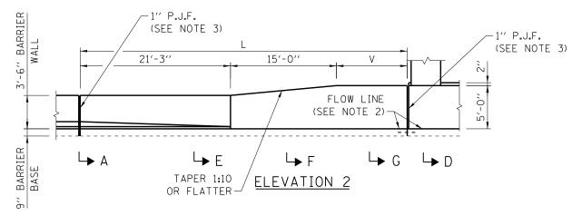
CONCRETE MEDIAN BARRIER TRANSITION, TYPE V-F AT BRIDGE PIERS (FOR W ≤4'-0")
