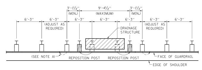
TYPE A GUARDRAIL - DRAINAGE STRUCTURE CONFLICT TWO POSTS
