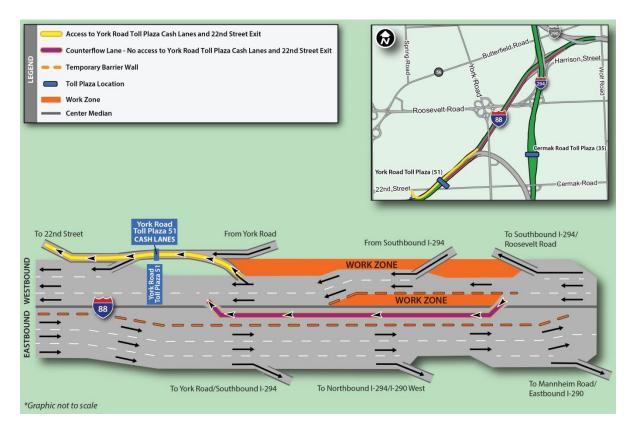
In late summer, a new traffic configuration will be put in place to complete reconstruction of the westbound lanes on I-88. At that time, the westbound lanes will shift to the right onto newly construction pavement. Eastbound traffic and the westbound lane traveling on the eastbound side will remain in the same configuration. Traffic is scheduled to remain in this configuration into winter. Reconstruction of the eastbound side of I-88 is scheduled for 2019.
