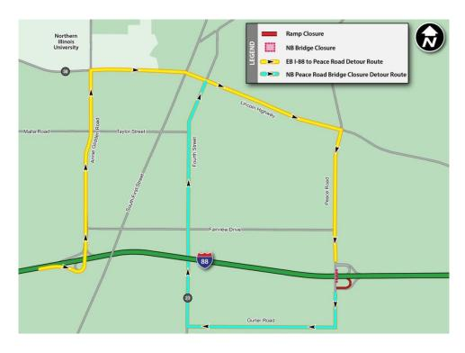
At the Peace Road Interchange, work is scheduled to repair all four ramps, including bridge deck and substructure repairs and installation of LED lighting. Ramp and bridge closures and detours will allow the Tollway to safely accommodate construction and will allow the work to be completed in half the time.
