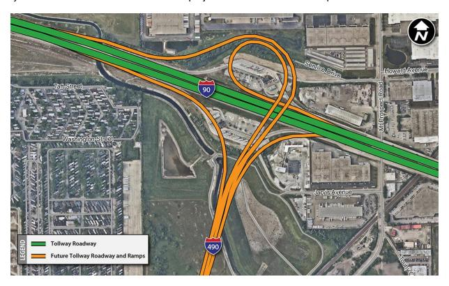
In 2018, advance work is beginning to prepare for construction of the new ramps and bridges that will connect I-490 to westbound I-90. Work will include construction of collector-distributor roads along I-90, retaining walls and barrier walls, as well as drainage and utility work. Closure and removal of the 7-Eleven fuel stations at the Des Plaines Oasis will be scheduled in early 2019.
