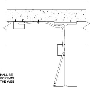
TYPICAL CONDUIT AND ENCLOSURE ATTACHMENT
