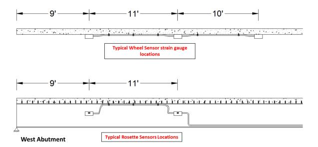
Fig. 4 Elevation view of the BWIM sensor locations
