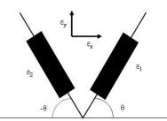
Fig. 2 Inverted delta shear strain rosette.
