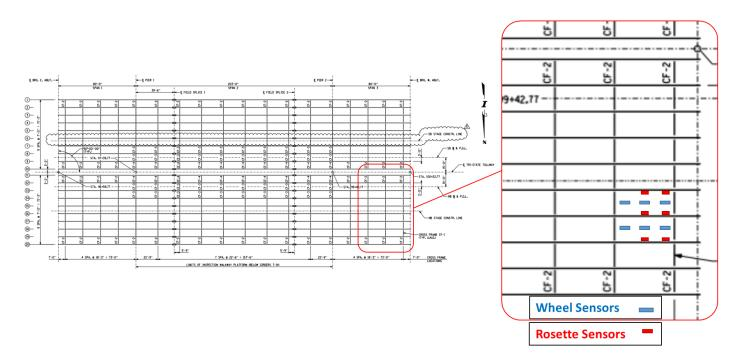
Fig. 3 The plan view of sensor locations, shear and wheel sensors.
