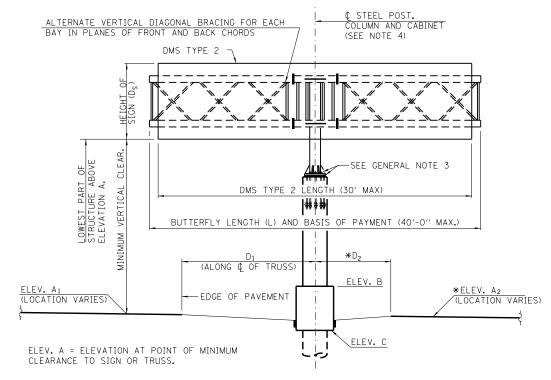
\* ELEVATION A2 AND DIMENSION D2 NOT USED WHEN BUTTERFLY STRUCTURE IS MOUNTED ON RIGHT SIDE OF THE SHOULDER. TYPICAL ELEVATION
