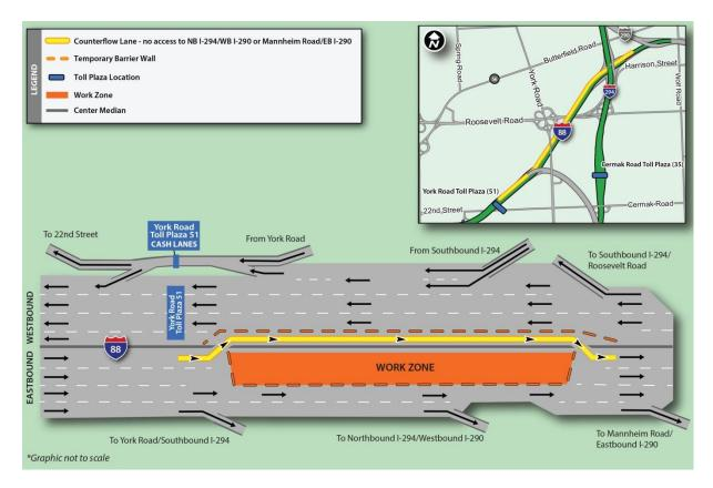
All work is weather dependent, and additional traffic shifts will continue as roadway construction progresses. Throughout construction, eastbound traffic traveling on the westbound side of I-88 will not have access to exit to the Tri-State Tollway (I-294) or to Mannheim Road.
