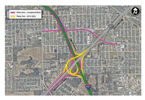
To complete the I-294/I-57 Interchange, four new ramps will be built connecting southbound I-57 to I-294 and 294 to northbound I-57. As part of this work, a new I-57 median will be constructed and the I-57 mainline will be widened. Work will also include excavation, drainage improvements, erosion control and new landscaping, as well as retaining wall, noisewall and bridge construction.
