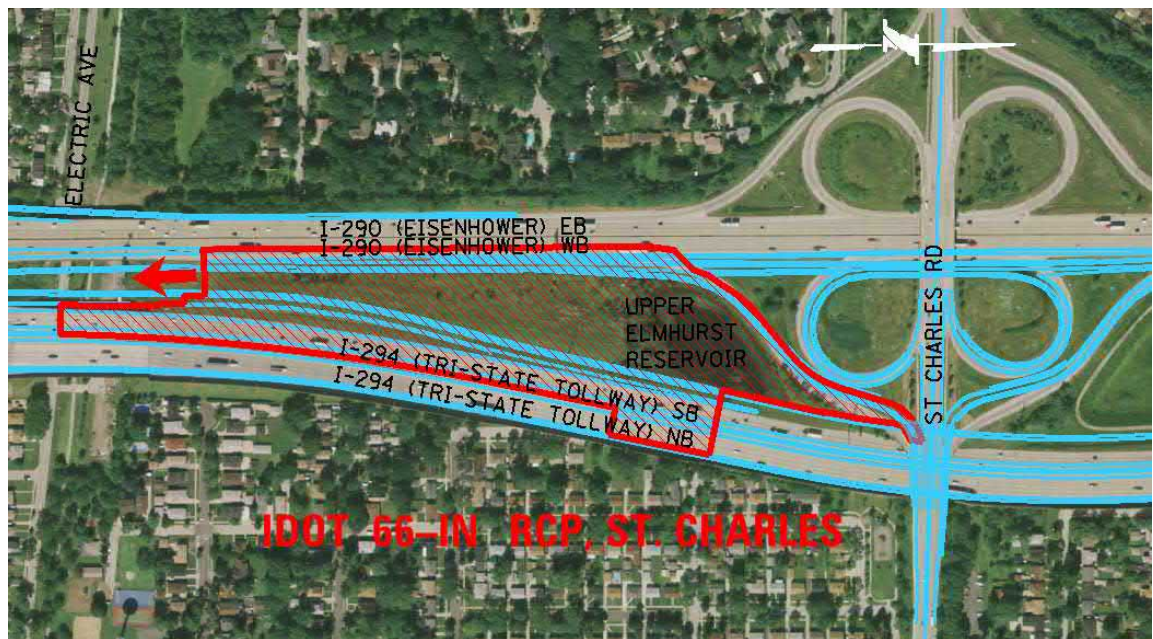
Figure 34: IDOT 66” RCP, St. Charles Drainage Area
