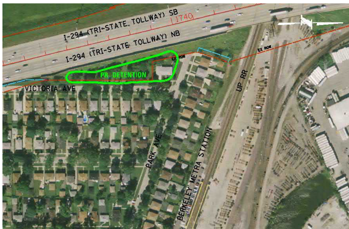
Figure 5: Berkeley Flooding Location and Proposed Detention
