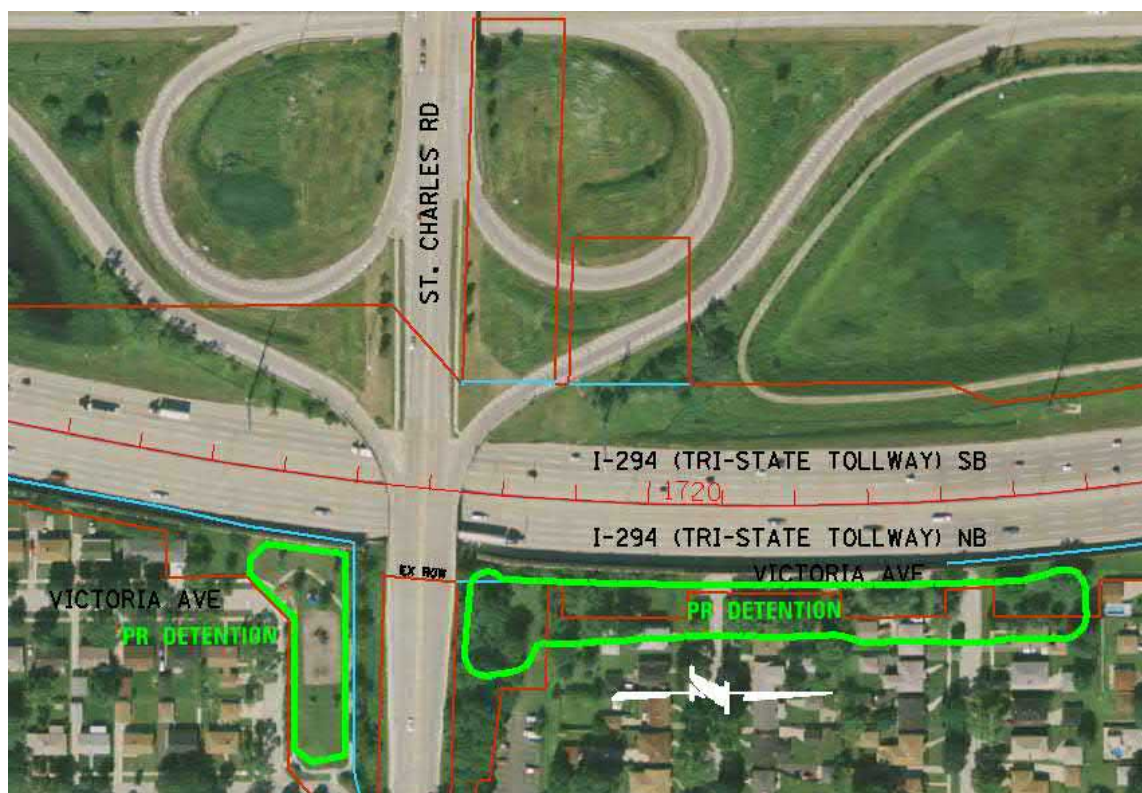
Figure 4: St. Charles Flooding Location and Proposed Detention
