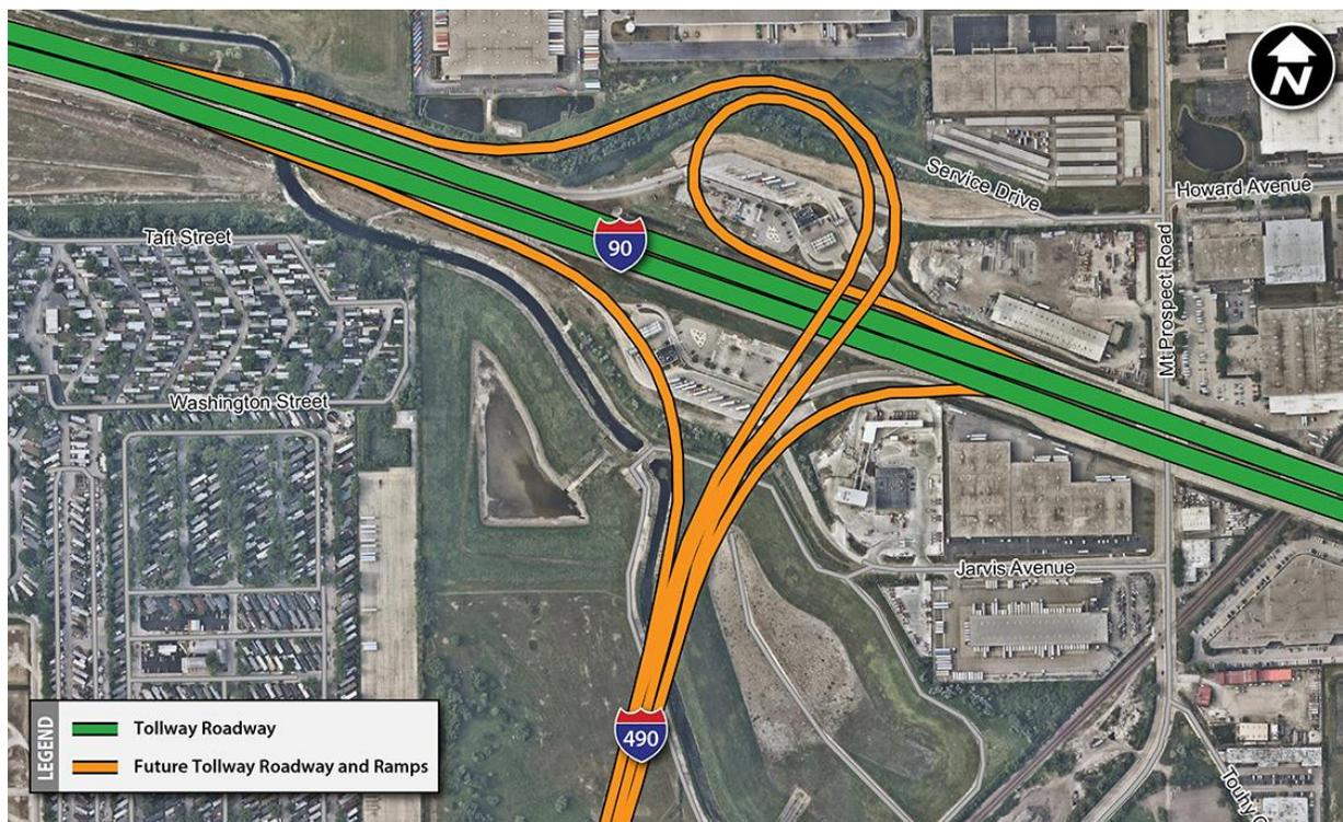
In 2018, advance work is beginning to prepare for construction of the new ramps and bridges that will connect I-490 to westbound I-90. Work will include construction of collector-distributor roads along I-90, retaining walls and barrier walls, as well as drainage and utility work. Closure and removal of the 7-Eleven fuel stations at the Des Plaines Oasis will be scheduled in early 2019.
