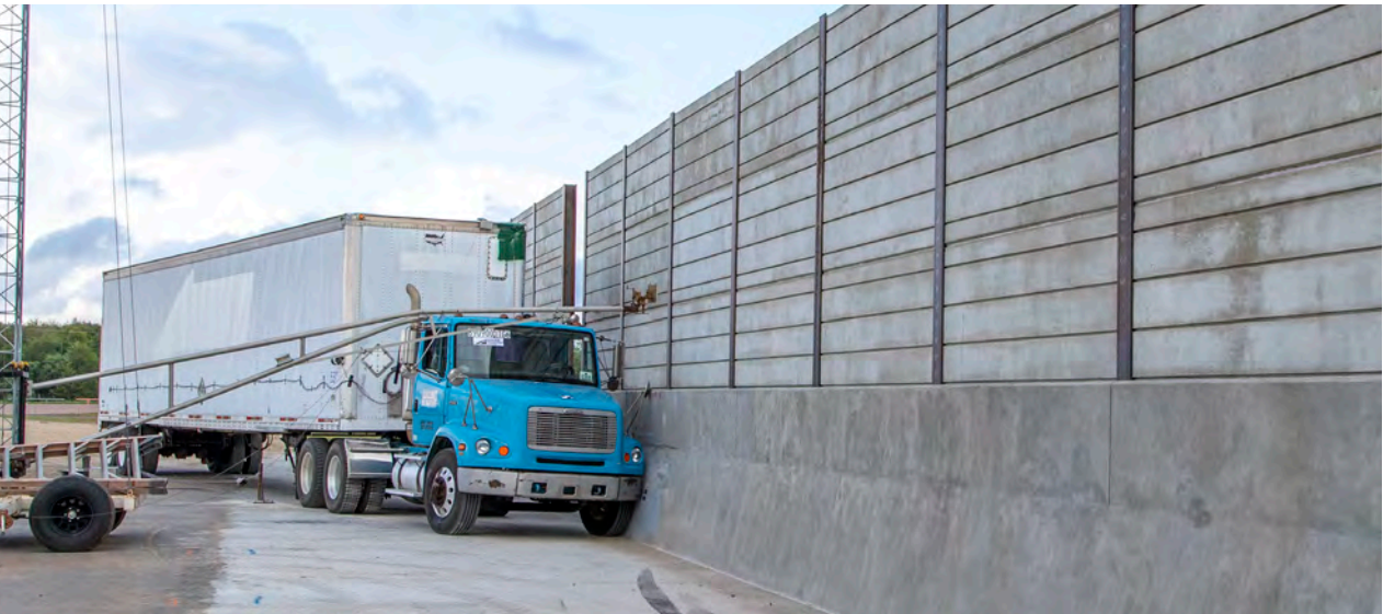
Pre-crash test staging includes tractor trailer with newly installed Constant Slope Barrier System at TTL.
