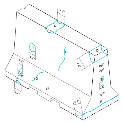
Above is a diagram of a temporary concrete barrier with some typical defects that may be acceptable. Below are the descriptions of defects that may be deemed acceptable.
