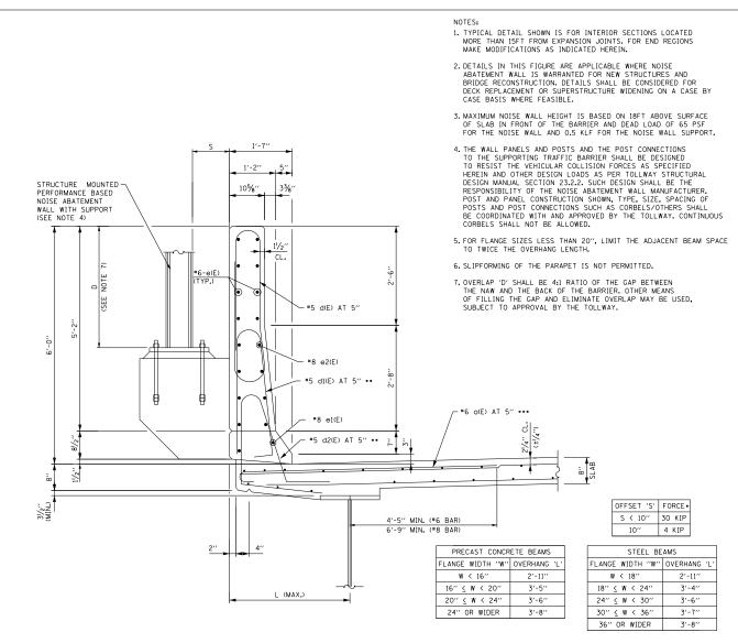
• VEHICLE COLLISION FORCE IS THE LOAD APPLIED TO THE NOISEWALL AT THE HIGHEST POINT UP TO 14FT ABOVE SURFACE OF PAVEMENT IN FRONT OF THE BARRIER. FOR AN OFFSET LESS THAN 10". THE FULL 30 KIP FORCE SHALL BE APPLIED TO THE NAW. OFFSET 'S' WILL BE DETERMINED BY THE NOISE ABATEMENT WALL MANUFACTURER.
